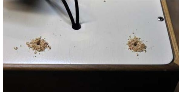
b) The speed box mounting holes are on its bottom. They are separated by 100 mm (10 cm). Use an awl or similar to mark the first hole. Then do the same 100 mm to the side to mark the second hole. Use a 1/8" drill to make the two mounting holes.
